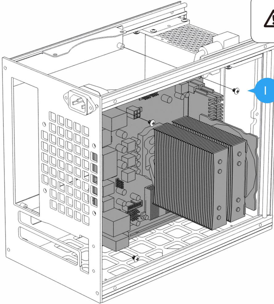
Highly recommend to install the CPU cooler and ram before installing the motherboard.
