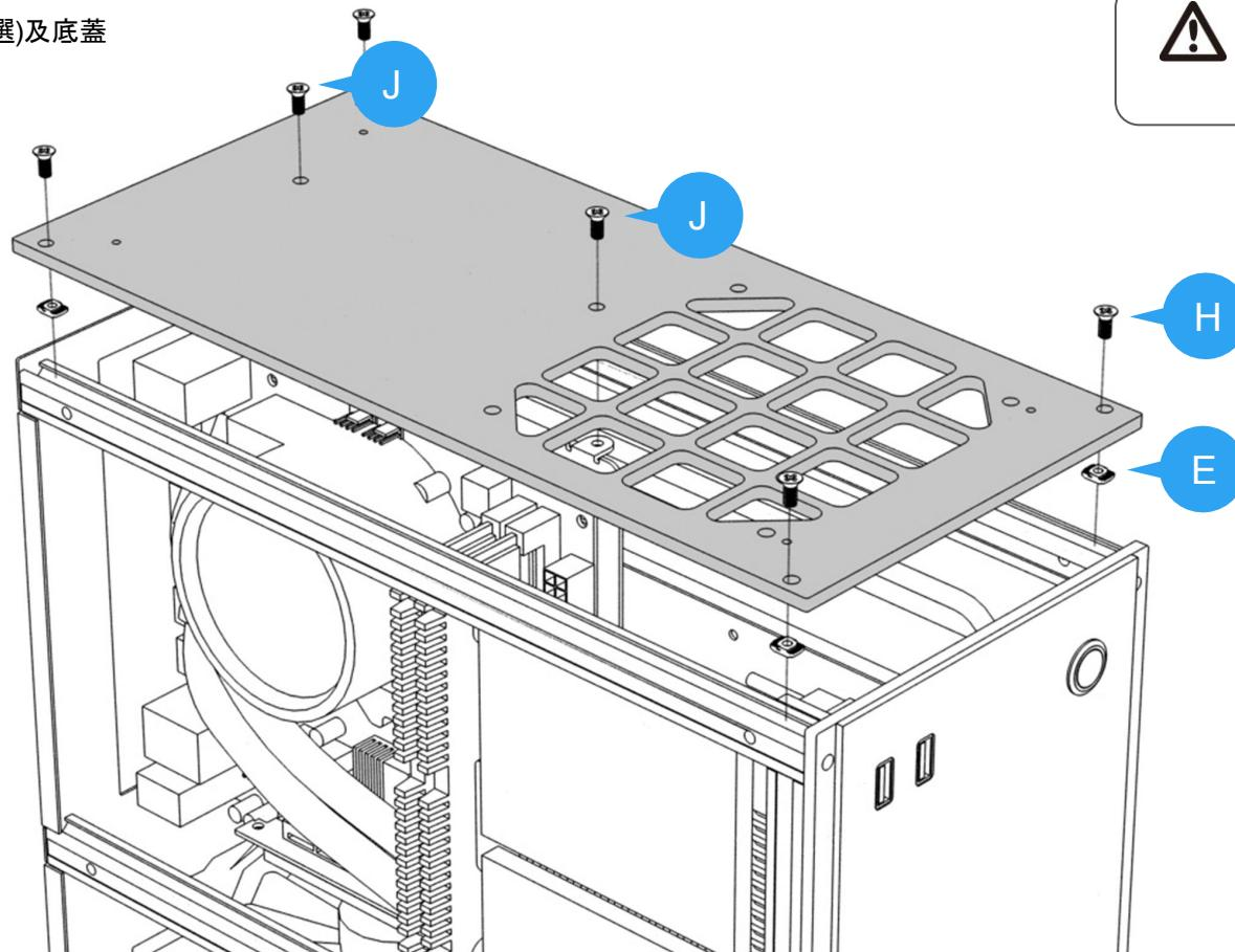
Please complete the cable management before installing the bottom panel.
