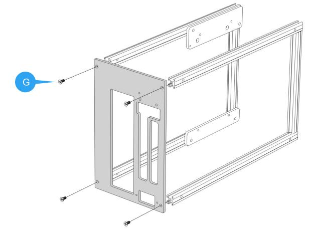
Install the PSU Metal Bracket on the Front Panel
