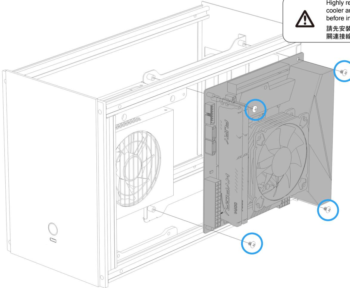
Highly recommend to install the CPU cooler and ram, power switch connector before installing the motherboard.
