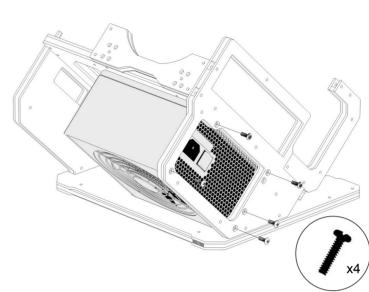
Step 7-2 : SFX, SFX-L PSU Installation
